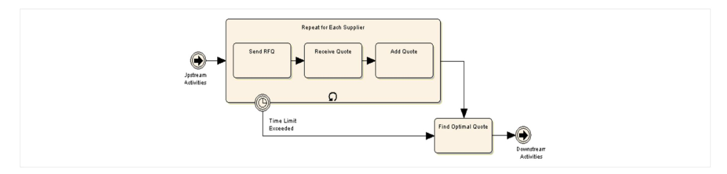
The above diagram illustrates a number of key features of BPMN, specifically the ability to create hierarchical decomposition of processes into smaller tasks, the ability to represent looping constructs and the ability to have external events interrupt the normal process flow.
