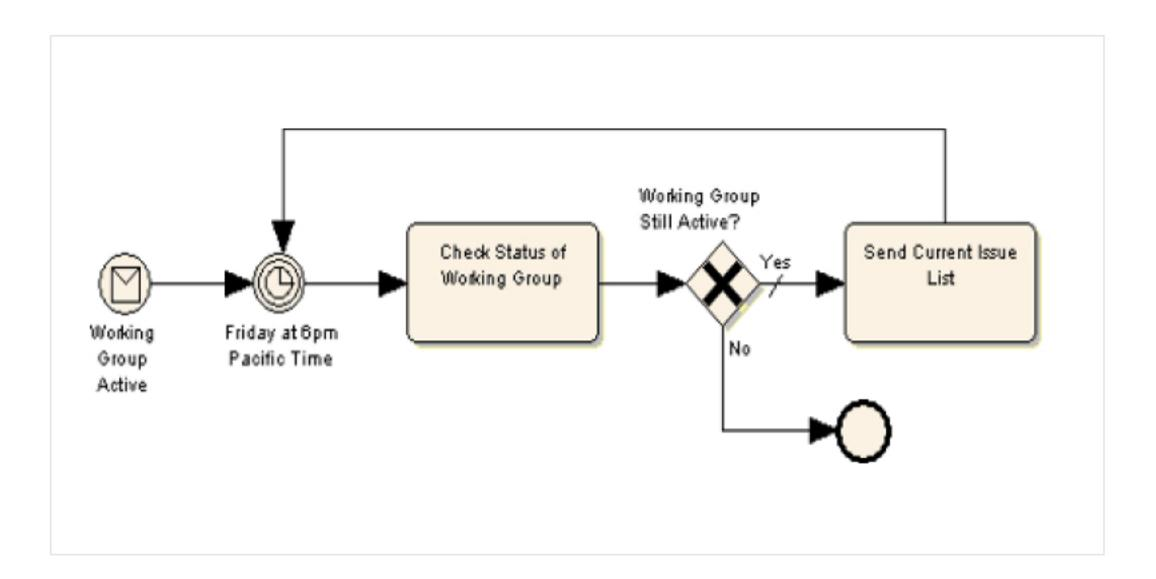
The above diagram shows a process being initiated by an event - in this case a message-triggered start event which notifies the process that the working group is active. The diagram also shows a loop being controlled by a timer event, and it shows a decision gateway (in this case, an XOR decision gateway) controlling when the loop is terminated.
