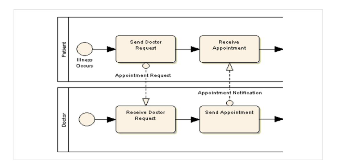
This diagram illustrates the use of pools to show interacting processes and the way that messages are passed between pools using message flow connectors.
